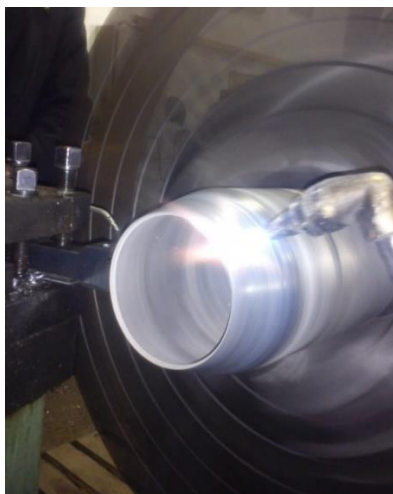
Fig. 6 Experimental configuration of tube spinning.
