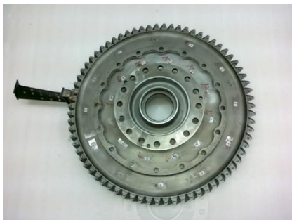
Fig. 3 Disc and a blade connected to it
